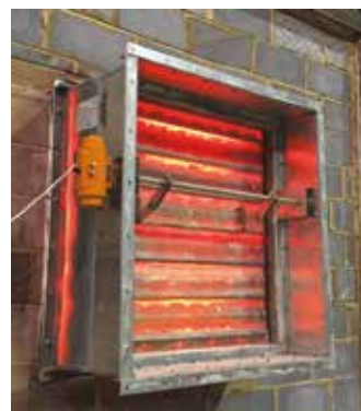
Damper Condition after 2 Hrs
