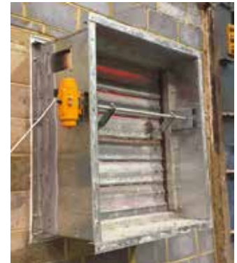
Damper Condition after 4 Hrs
